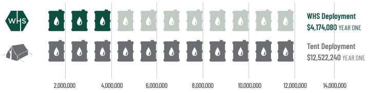
Assumptions: 1000 man camp tent deployment uses 9 generators of 240kWh running at 3/4 load. First year savings higher due to equipment cost, \$1.8M for 9 generators vs. \$600K for 3 generators. 1000 man camp WHS deployment uses 3 generators of 240kWh running at 3/4 load| Fuel costs \$10/galTent
